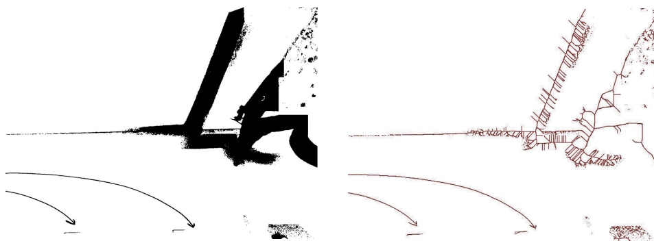
Figure 7.6: Upper right quadrant of sample picture (left: input to skeletonizer, right: output of tracer)
